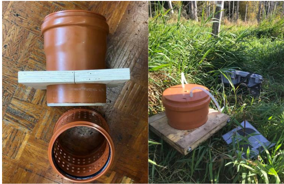
Figure 25: Soil chamber upper and lower part on the left and on the right the measurement of the gas flux in the wet soil in mid-October (own photo, 2022).
