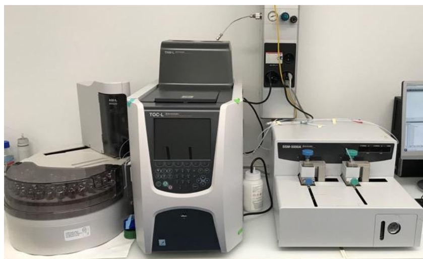
Figure 19: Measuring instrument at EAWAG for the determination of TOC and DOC in water samples (own photo, 2022).
