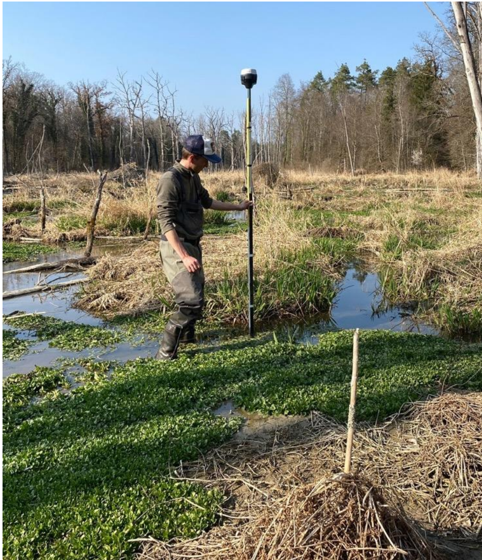
Figure 16: GPS recording and reading of water depth in the middle pond to calculate the volume of water stored in the study area (photo courtesy: Carlos Pinto).
