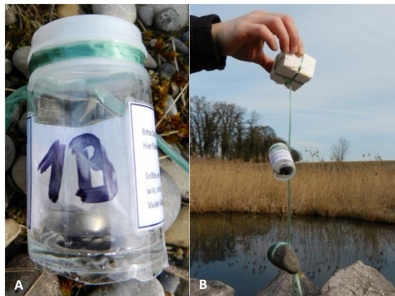
Figure 7. Pictures of the data logger buoy system used for the temperature measurements. A shows the glass tube carrying a Thermochron® iButton logger. The logger was put into a water proof, resealable plastic bag and the glass tube was sealed with Parafilm®. B: The glass tube is fixed 15 cm under the styrofoam buoy and charged with a stone to hold it at the correct position under water. A tent peg or stone anchored the construct to the ground to hold it in position in the pond.
