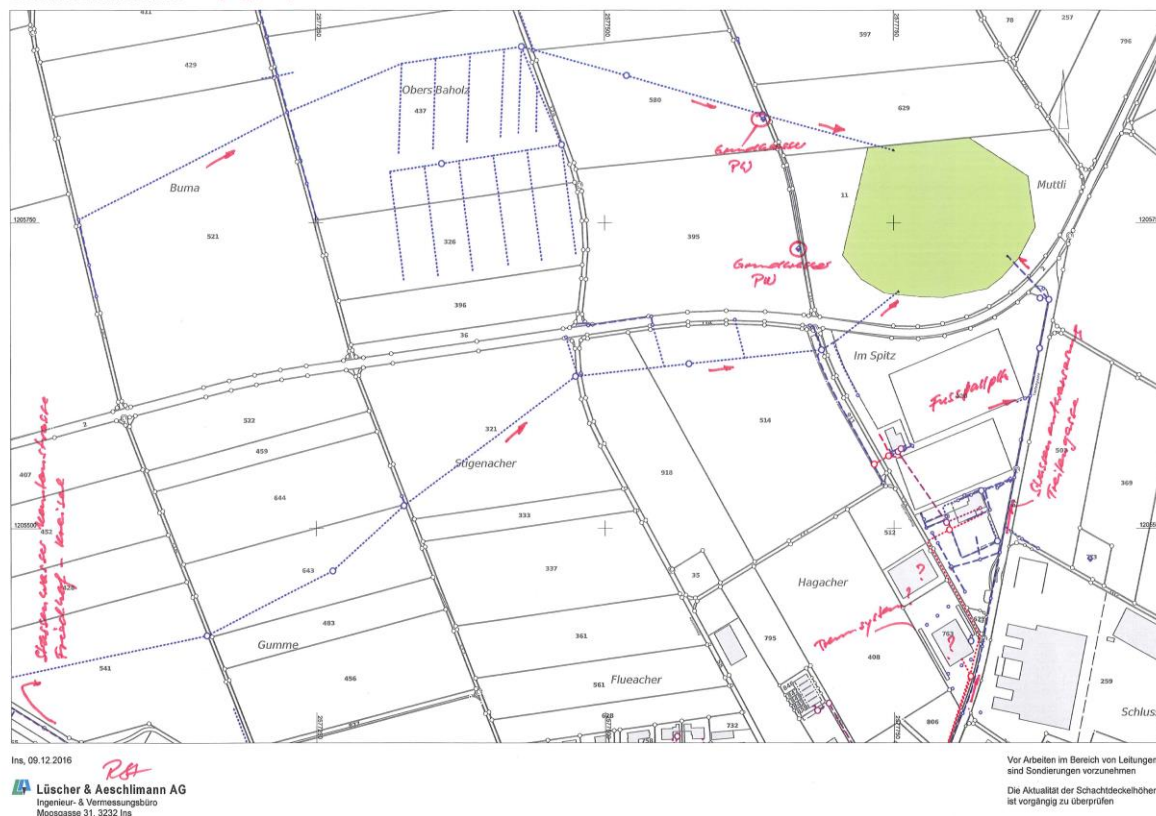
Figure 12: Drainages in the surrounding of Muttli (1:8000). The red arrows indicate, in which direction the water is flowing.
