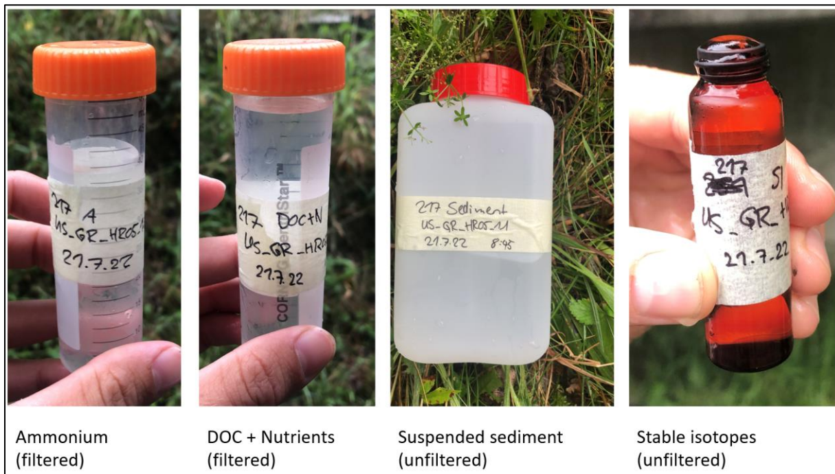
Figure 21: Four types of water samples. In winter DOC and nutrients were in separate falcon tubes. Ammonium and DOC + Nutrients samples were filtered with a 0.22 \mu\text{m} filter.
