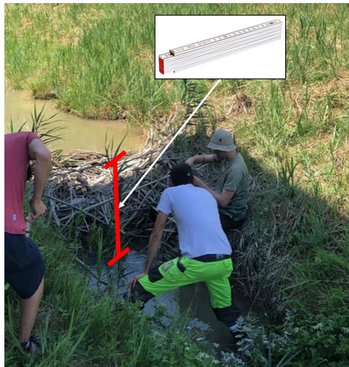
Figure 25: Measurement of dam height. Raphael filtering the water samples, Owen registering the dam location and Mael measuring the beaver dam height with a meterstick (from left to right).
