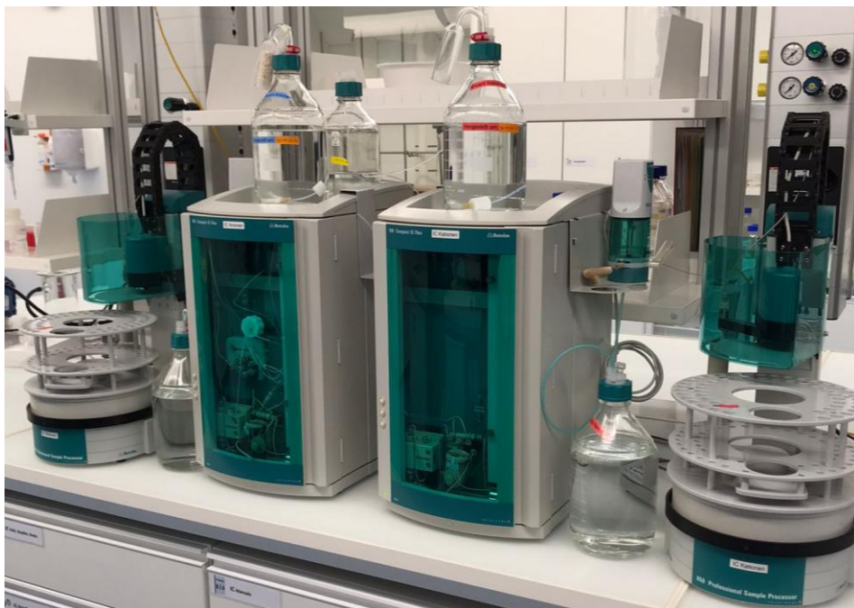
Figure 27: Metrohm 930 Compact IC Flex. Measuring device at EAWAG for the nutrient samples.
