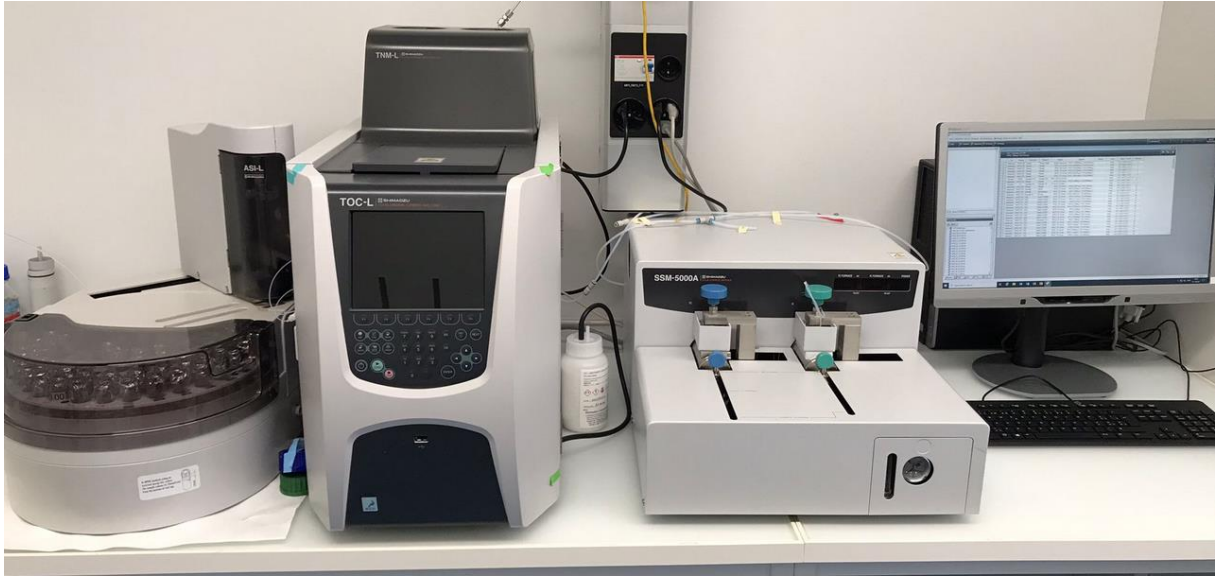
Figure 28: Shimadzu TOC-L CSH. Measuring device at EAWAG for DOC.
