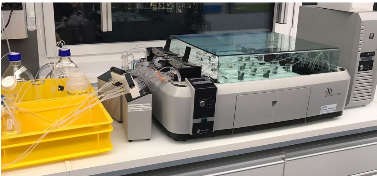
Figure 29: Skalar San++ Autoanalyzer. Measuring device used at EAWAG for ammonium analysis.
